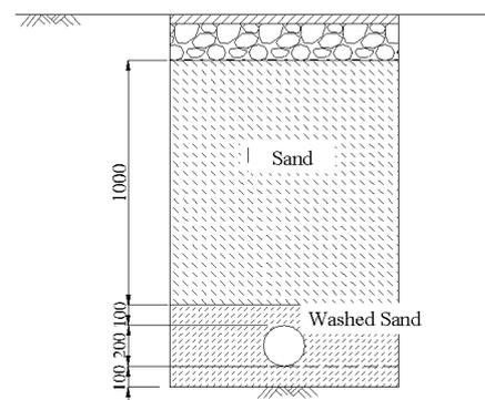
Figure 4 Liquefaction countermeasure for drainpipes in farming villages
