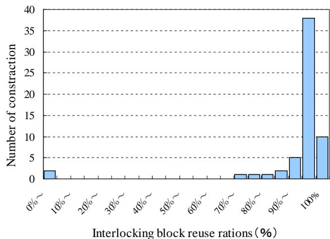
Figure5 Interlocking block reuse ratios at about 60 sites in around Sendai City
