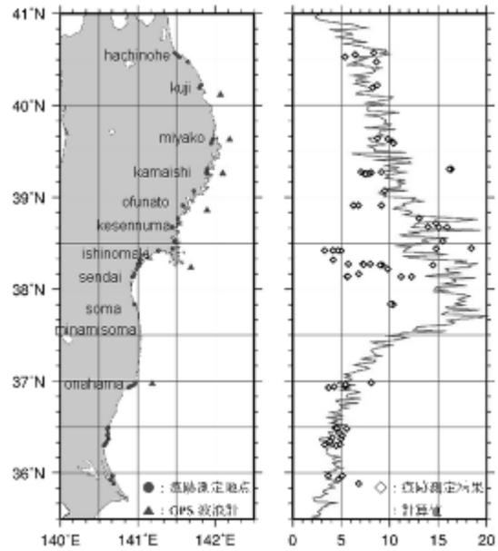
Figure 2 Measured and calculated run-up heights of tsunami
