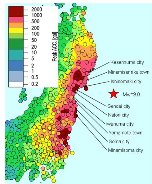
Figure 1: Measured peak ground acceleration, and locations of the survey areas
