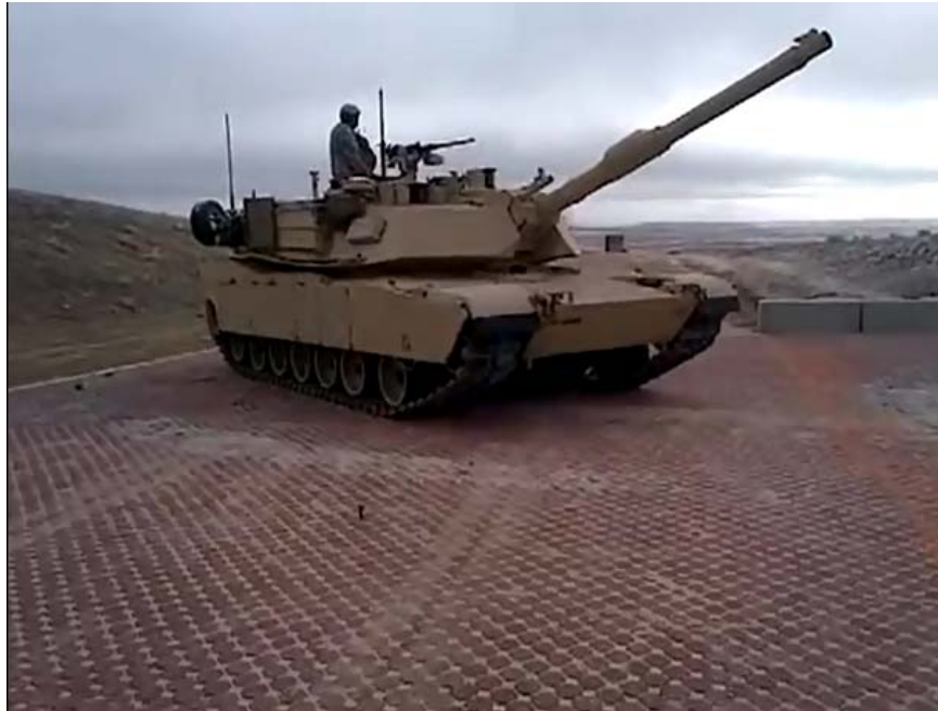
Figure 4. M1A1 Abrams tank on the permeable pavement test section.
